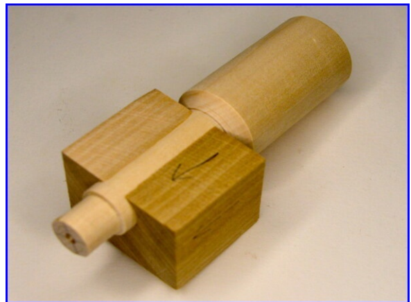
George Rodgers - Amana Colony Bench Maple, Cherry - Waterlox Tools for Setting Tapered Legs
