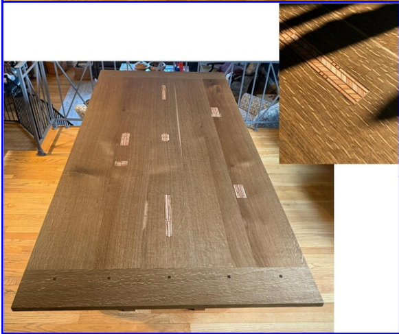
Bill Hoffman - Dining Table Quarter Sawn White Oak, Maple, Walnut Ammonia Fumed, OSMO Oil
